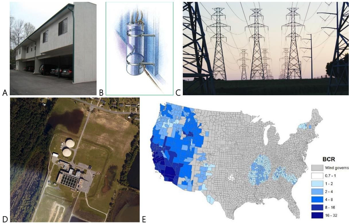
**Figure 2-2.** Five high-BCR mitigation measures that save at least \$30 per \$1 spent, some over 50:1: (A) soft-story retrofit, (B) securing residential water heaters to the building frame, (C) undergrounding high-voltage transmission lines, (D) adding a berm to protect a water treatment plant, and (E) building-code development since 1990.
