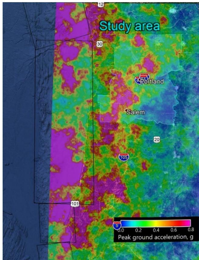
Figure ES-1. Cascadia Subduction Zone (black rectangles), study area (highlight), and one of 100 simulations of peak ground acceleration (color overlay)
